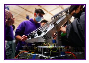
Throughout the week, electrical and mechanical worked hard and with great effort, making sure to put in the necessary time and effort to finish the practice bot. Mechanical was able to successfully complete the machining and assembly process for all the necessary parts. Meanwhile, electrical was able to install an igus chain on the elevator, and successfully finished wiring the bot.
